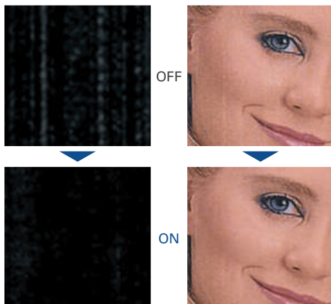
Problems such as nozzle misfire and streaks are detected and images automatically corrected by inline sensors.
