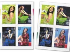
CMYK and RGB+gray(3C) are alternately printed on the margin of the printed sheets. In addition, registration marks are automatically printed on both sides of the sheet to check registration
